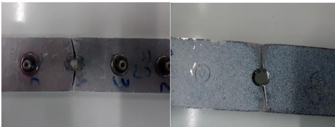
Fig.13: Top and bottom view of the failure.
