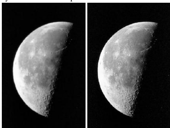
Fig.2: Before and after Laplacian filter application.
