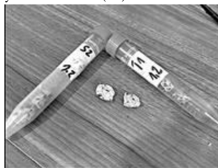
Fig.4: Fragments packaged for porosimetry and microanalysis assay.
